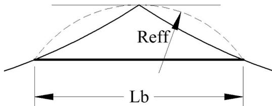
Rail stress arises from a number of factors but, if rails are expected to bend to follow the alignment of the bridge decks, the stress due to rail bending is in addition to the stresses normally experienced in service.
