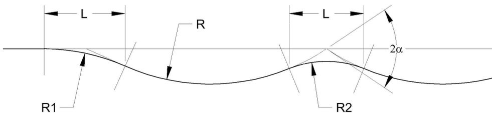
Using a CESuRa joint the track can be arranged with a series of reverse vertical curves.
