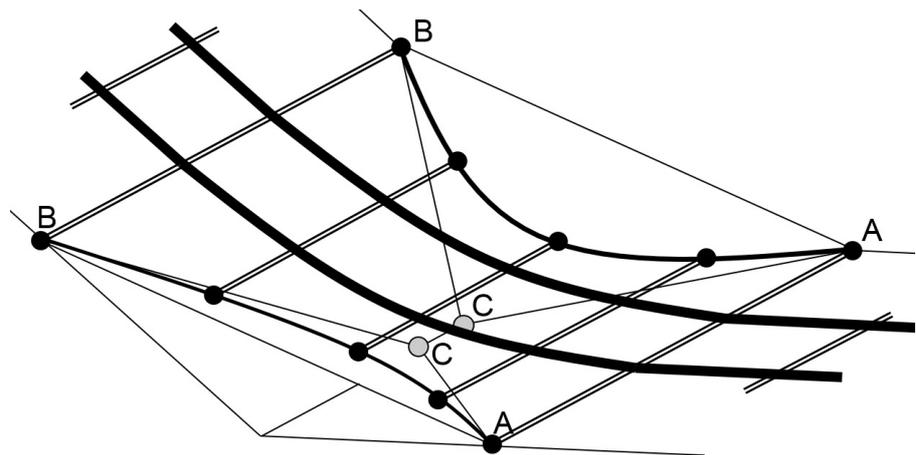
Real applications introduce complicating factors, for example the height of bearings and the wings and bearer bars causes rail dilation. Also the central bearings C may have to sit on one side or the other of the hinge, however provided they are reasonably distant from the spine AB and located along the lines AC or BC the above relationships hold.
