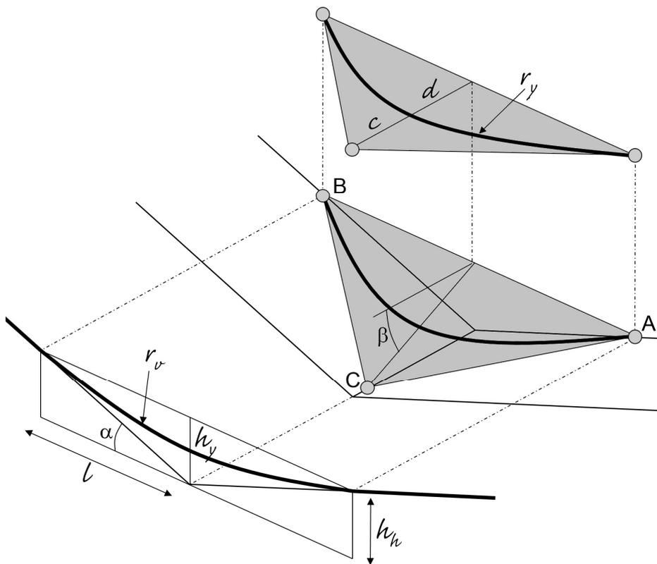
The wing rotates through an angle  $\beta$  and then the projection of the radius of the yoke on the vertical plane takes up a radius  $r_v$ . It is this radius that determines the permissible speed.
